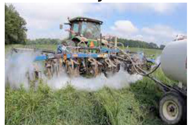
Grower applying anhydrous ammonia with his tractor, applicator, and pulling the long white storage tank. Submitted photo
