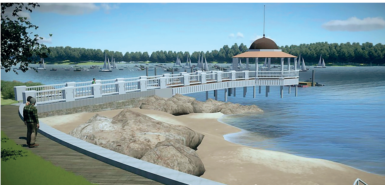
There were three options for renovating the Rotunda to meet new federal standards for tide surges, but in the end the Select Board voted for Option 1, seen here, in which encased steel pilings would raise the structure to 19' on its current footprint, costing $2.3 million. Image: Foth Engineering 2023
