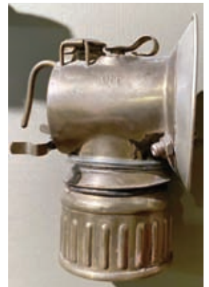
Above: This carbide lamp burned acetylene, produced by dripping water on to calcium carbide. Left: This large, German-made lamp burned acetylene.
