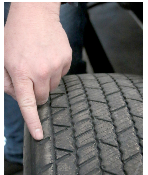
Mitch Morris shows where he grooves and sipes tires between treads to improve grip.
