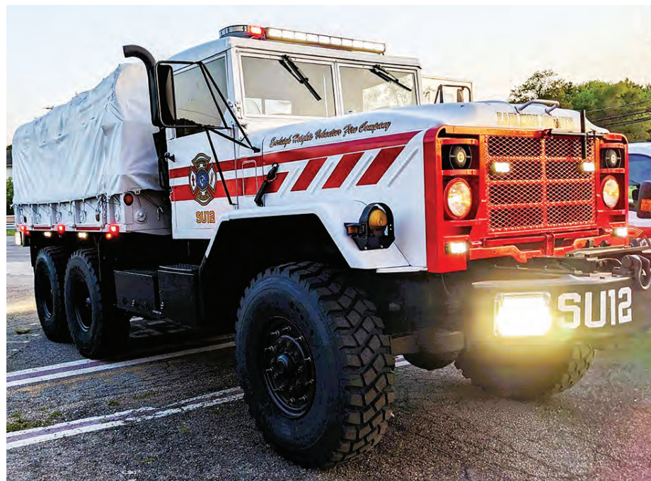
The truck can ford through floodwater 36 inches deep and operate in deep snow.
